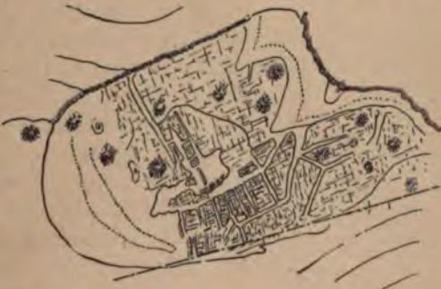
FIG. 190. — Sketch map of the Oucane de Chabrières near Chorges in the High Alps, to illustrate the corrosion of limestone along two series of vertical joints (after Martel).
